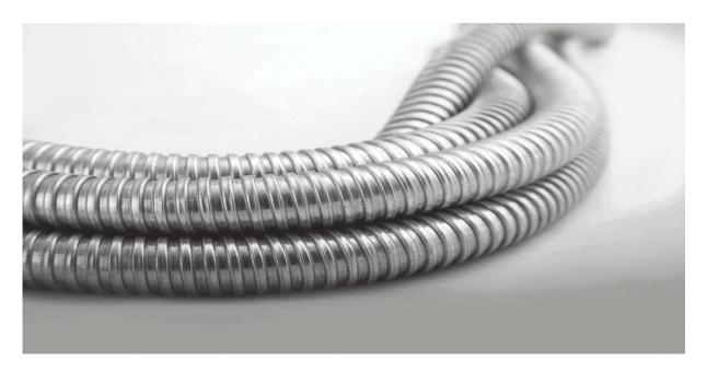
Galvanized steel flexible conduit is suitable for concealed, exposed or approved raceways. The flexible conduit is manufactured with a continuous spiral wound strip of corrosion rust resistant, hot dipped galvanized steel.
